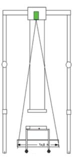
This sensor measures the position of this beacon and calculates the lane number, the X position on the long side of the lane and Y position on the transversal side of the lane (position used for checking).
