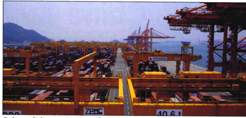
Seoho supplied automation systems for 36 twin cantilever RMGs at HPNT in Busan
