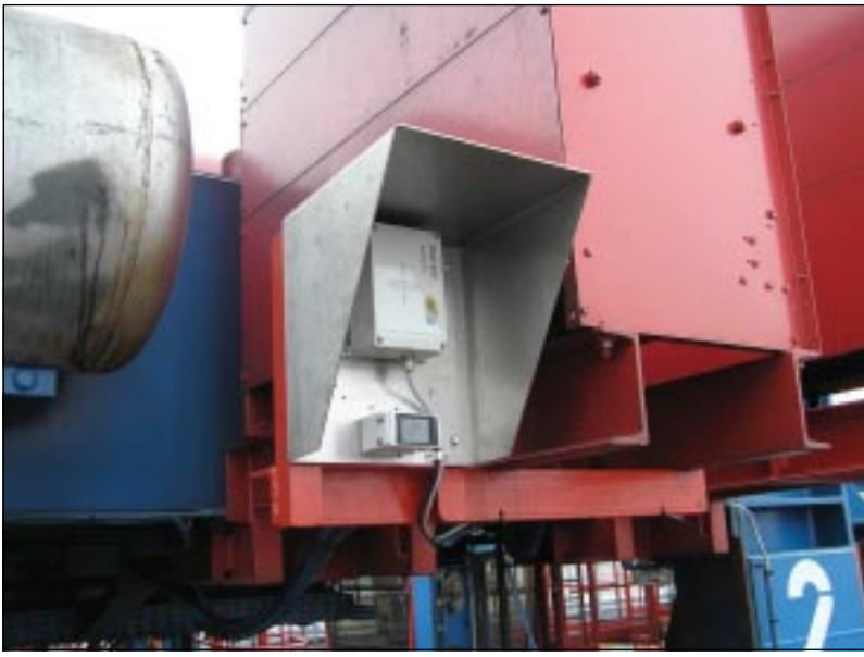
Micas frequency modulated continuous wave radar sensor in a collision avoidance application on a straddle carrier
