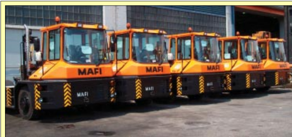
The Greek Port of Piraeus has been supplied with 12 new Mafi ro-ro MT 30 F tractors, with the purchase conducted by Athens-based D F Sarantopoulos SA. The main features of the new tractors include 4 x 4 drivelines, incorporating the latest 174 kW Volvo engine model TAD 720 VE and the ZF 6 WG 200 gearbox type. The cabin is integrated fully with ROPS and meets the latest safety standards. Additional features include a fully automatic A/C unit designed for driver comfort as well as an air suspended rear axle, a Eurohitch-Holland fifth wheel plate and the newly-conceived swivel seat console. The Port of Piraeus has stated that low maintenance and service costs were a major contributing factor towards their decision for choosing Mafi
